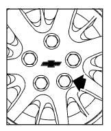
To remove the steel wheel covers and wheel nut caps, loosen the plastic nut caps with the wheel wrench in a counterclockwise direction. If needed, you can finish loosening them with your fingers. The plastic nut caps will not come off.
